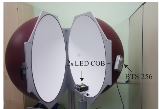
Fig. 4. Integrating sphere with BTS256 with cone measuring adapter.
