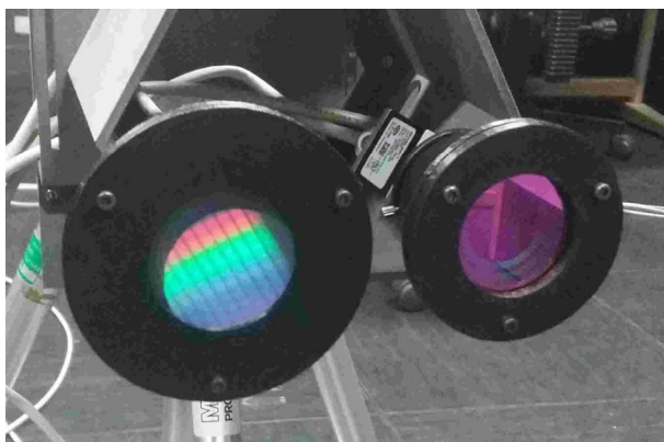
Fig. 3. The multi luminance meter (on the right) and the multi-spectrometer (on the left)
