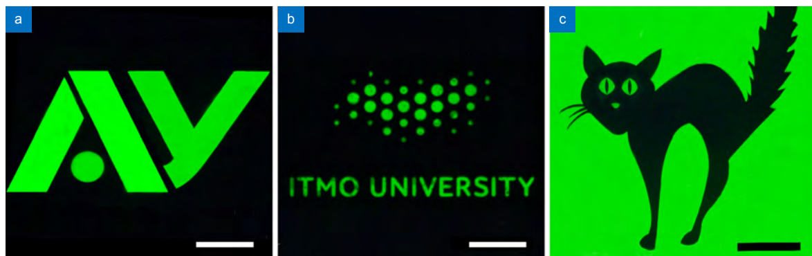
Fig. 7 | Optical images of our n^{+} -Si(100)/CsPbBr 3 :PEO:LiTFSI/SWCNT mat devices in shape of. (a) Alferov University (Saint-Petersburg, Russia) emblem. (b) ITMO University (Saint-Petersburg, Russia) emblem. (c) Inverted composite perovskite cat. Scale bars in all images are 500 \mu m.
