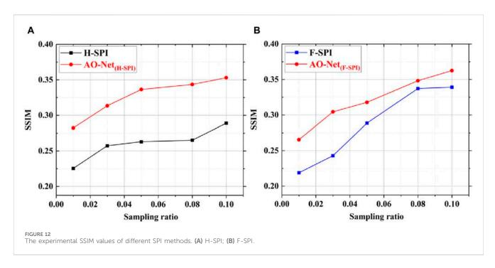
image. The above results showed that AO-Net can achieve higherquality imaging at low sampling ratios. Therefore, combined with simulation results, we could choose the appropriate basis patterns according to different application scenes to ensure maximum efficiency.
