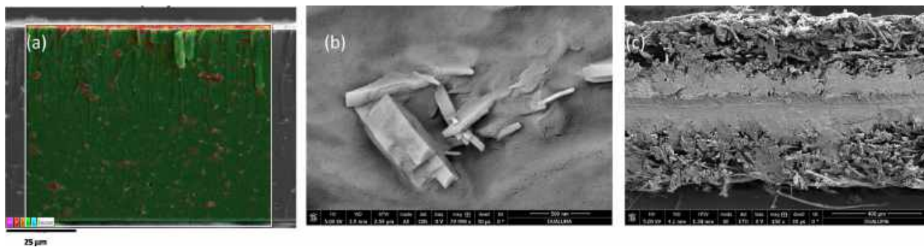
Figure 5. SEM images for N/Tb-II membrane: (a) cross-sectional SEM–EDX, (b) surface FE-SEM, and (c) cross-section of MEA after conducting the fuel cell durability test.
